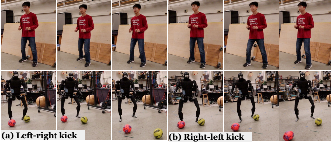
Fig. 5: The humanoid robot is able to track the precise lower-body movements of the human teleoperator.
