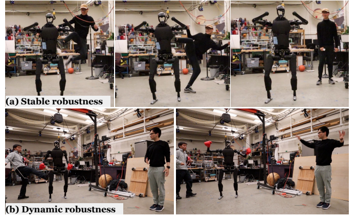
Fig. 7: Robustness Tests of our H2O system under powerful kicking. The policy is able to maintain balance for both stable and dynamic teleoperated motions.
